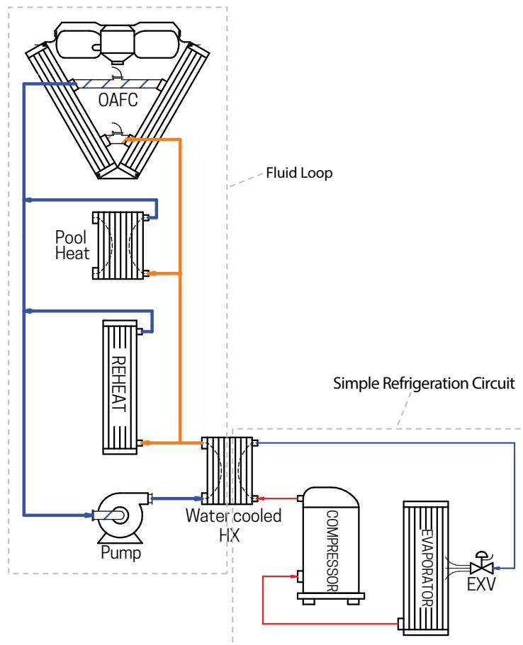
Fluid cooled systems have significantly lower refrigerant charges and as a result dramatically reduce carbon emissions. The principle is simple: liquid is a more efficient heat transfer medium than air, allowing the system to operate at lower temperatures and reducing the workload on the compressor. This results in lower energy consumption as well as longer compressor lifespans.
