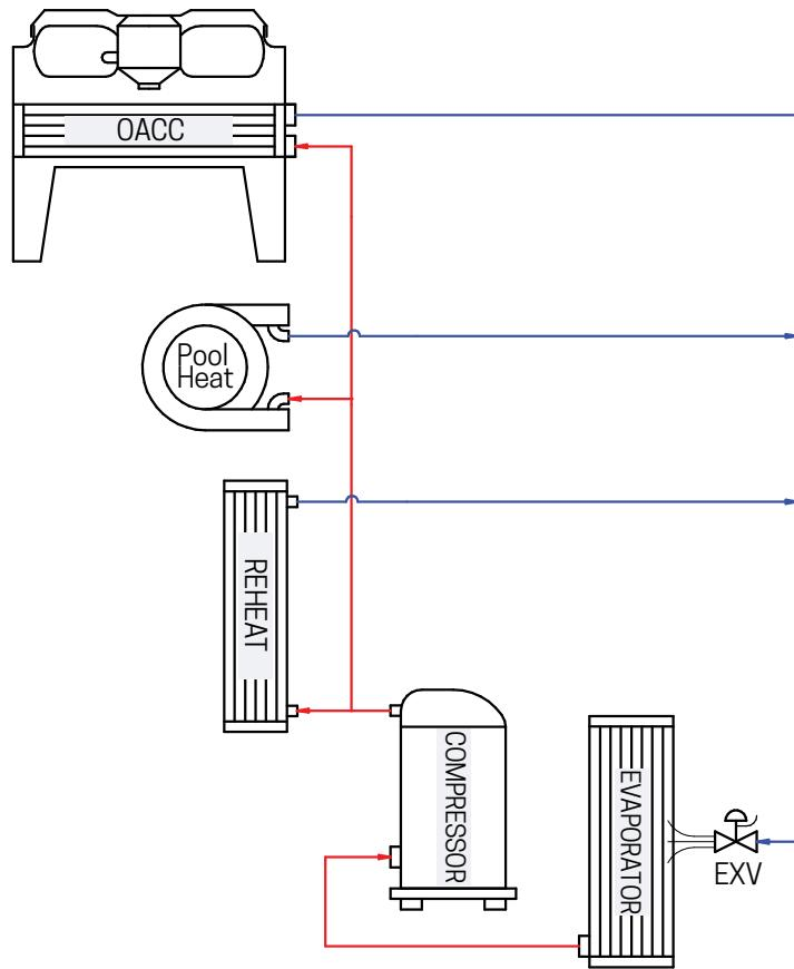
An outdoor air condenser sends refrigerant directly outside, where it is cooled and condensed by the outdoor air before returning indoors to absorb more heat.
